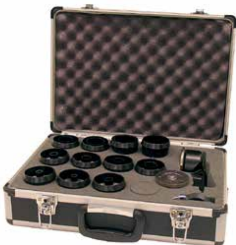
A case with 5 nozzles for pipes (6–42 mm)
